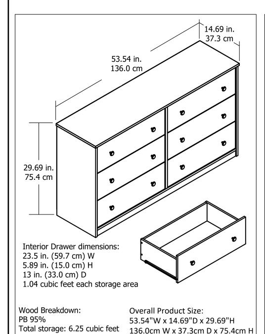
75 lbs. 34 kg 25 lbs. 11 kg (each drawer) **Maximum Weight Capacities** Unit Weight: 102 lbs. (46.3 kg)
